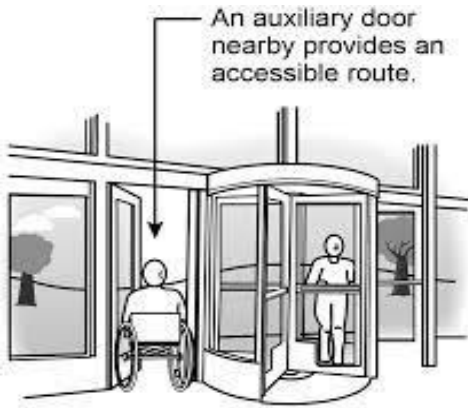
Auxiliary Door at Inaccessible Revolving Door
