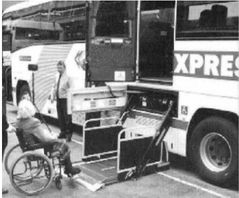
Photo 1. Hydraulic lift mounted at the bus entry
